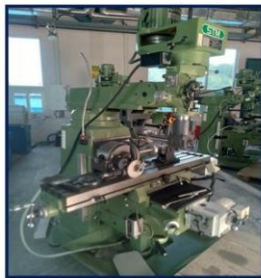
Vertical milling machine with Horizontal Set-up for Gear cutting
