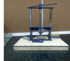
Spring Stiffness measurement set-up
