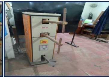
Spot Welding Machine
