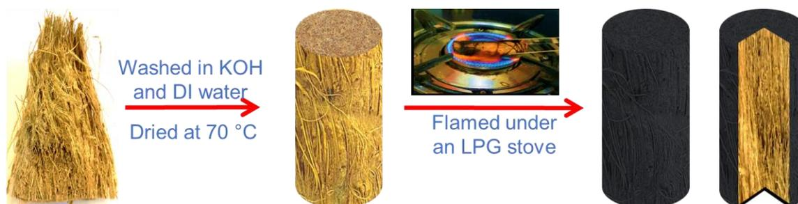
**Figure 4.1.** Photographs showing stepwise fabrication of FCH-based evaporator.
