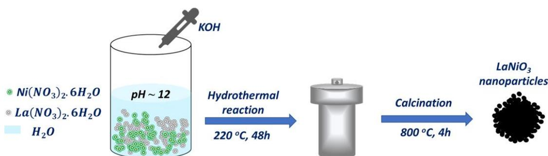
**Figure 5.1.** Schematic illustration of the hydrothermal synthesis of LNO NPs.
