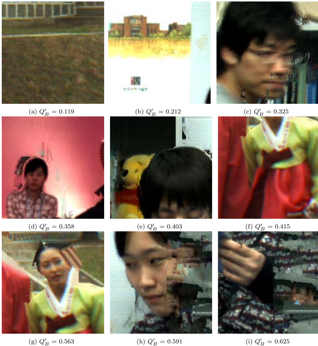
Figure 3.4: Examples of image blocks from the IETR dataset of different perceptual quality along with the quality score ( Q'_B ) obtained by the proposed NR model. Higher values of Score indicate poor perceptual quality.
